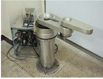
Fig. 4. Photograph of the 2 DOF mechanical system used in simulation and experimental studies.
